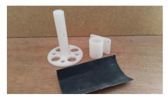
You may need to <u>lightly</u> sand the plunger shaft and runner for a smooth operation.
