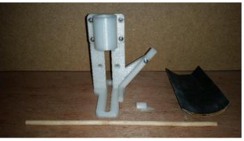
Ensure that the wood arm is fully seated into pivot arm and pointer. You can glue this together, I recommend using an epoxy for this.
