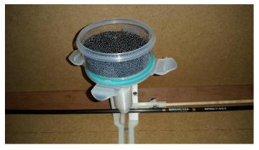
**Stage 9:** If you do not have an accurate scales to make your weight simply zero the scales with a carbon arrow of a known spine then add lead shot until the scale reads correctly for this arrow. (As carbon arrow spines are very accurate this method works well)
