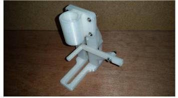
**Stage 3:** Arm assembly. You may need to lightly sand wood arm ends to fit snuggly into pivot arm and pointer end.
